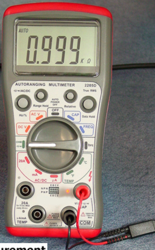
Resistance Measurement with 1K@1% Metal Film Resistor
