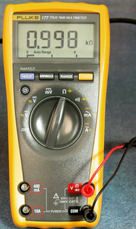
Resistance Measurement with 1K@1% Metal Film Resistor
